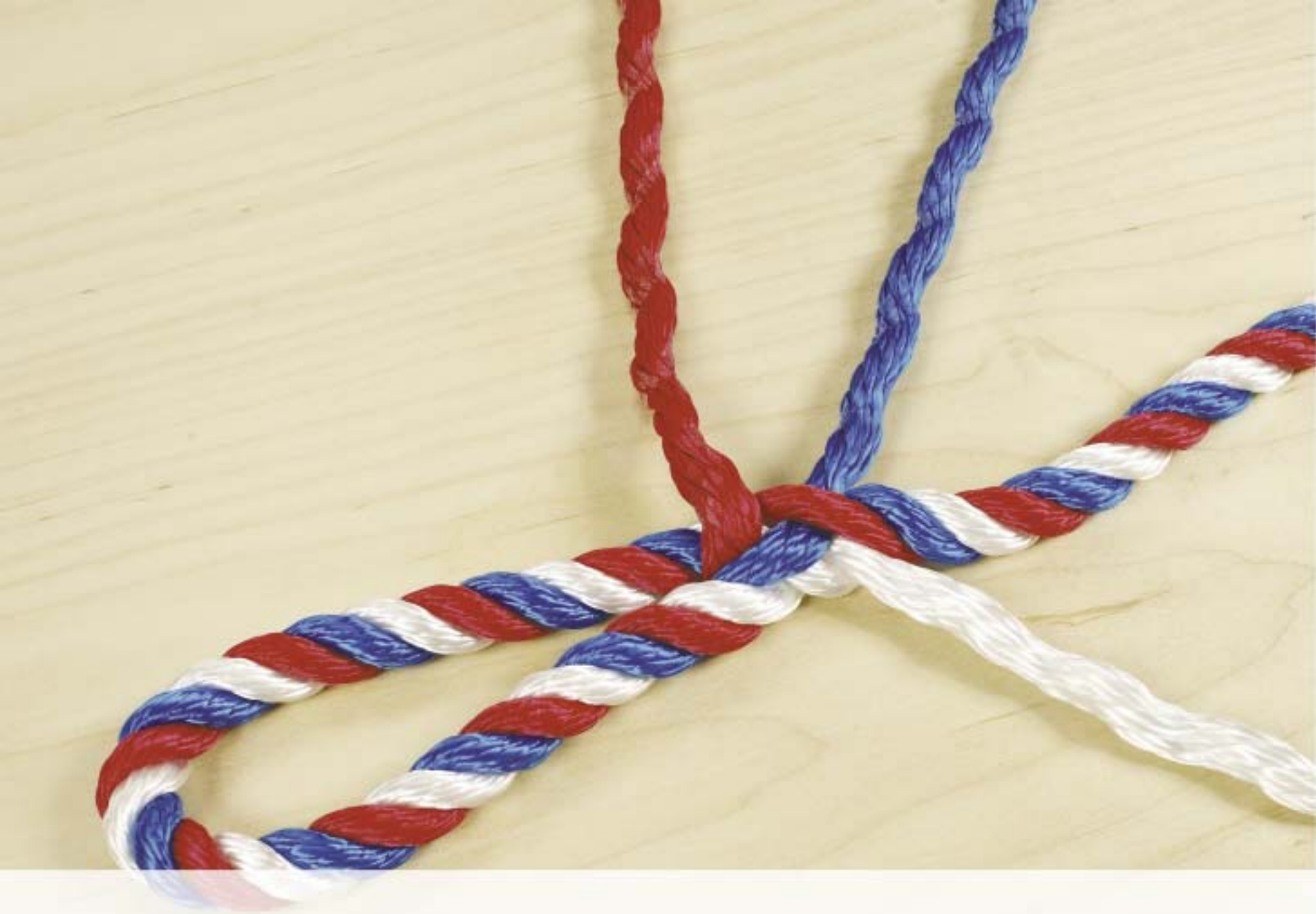
Photo showing the second strand pulled through.
